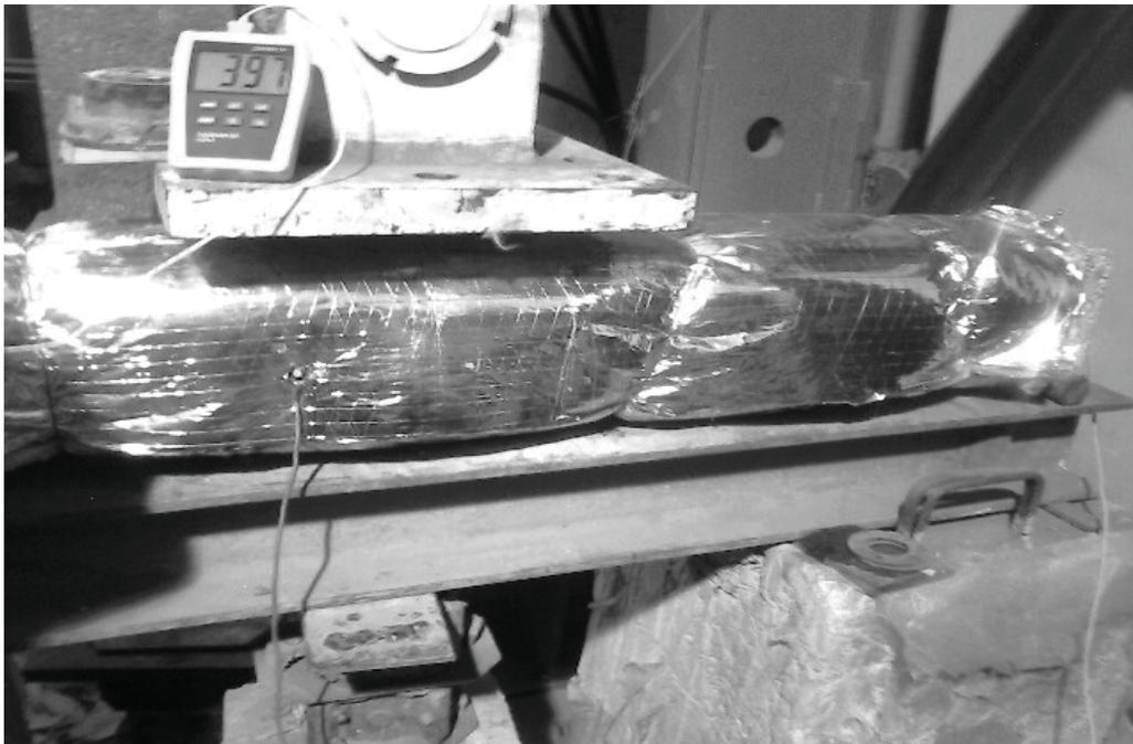
**Photo 2:** The heated beam upon reaching 397°C
