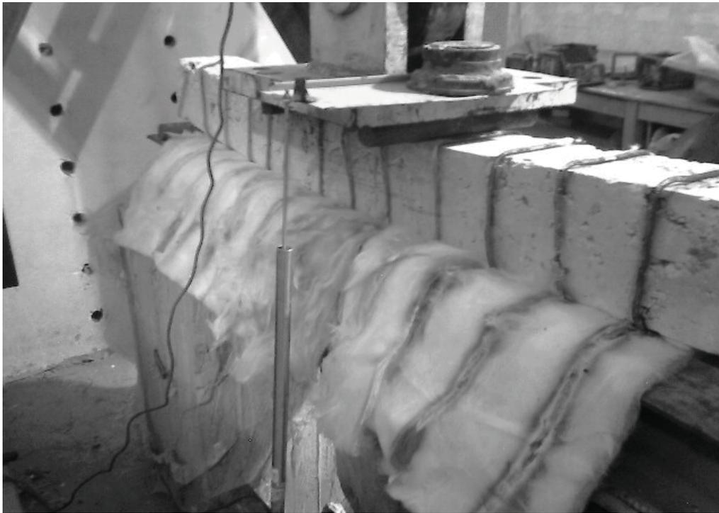
**Photo 1:** Technique of heating the RC beam and measuring displacement using LVDT
